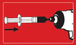
**4.** Inject grease into the anvil grease hole. Wipe away excess grease.
