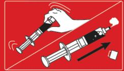
While holding the front of the applicator, shake it to move trapped air to the front. Remove the applicator cap. Push the plunger forward slowly to release air.
