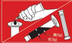
2. Fill to the tool specific mark:"1" (3g) for NC-4650H, "2" (5g) for NC-4233QH & NC-4255QH. Insert the plunger. Do not remove the applicator cap at this step.
